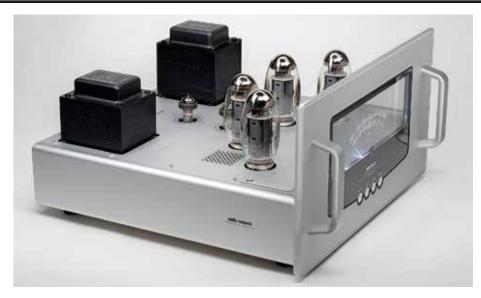
**ABOVE:** Factory-matched and held in check by ARC's auto-bias regime, the two pairs of KT150 tubes are fan-cooled once the lid is in place. Two custom-made transformers are fitted – one for the PSU with three secondaries [furthest] and the other with two primaries and three speaker output taps
