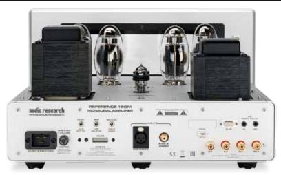
ABOVE: Small toggles switch between single-ended (RCA) and balanced (XLR) inputs, fan speed and auto-shut off (signal sensing). Tube hours are indicated beneath while 4mm speaker binding posts offer 16ohm, 8ohm and 4ohm-tapped outputs
