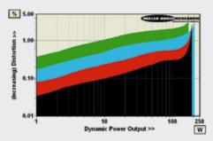
ABOVE: Dynamic power output versus distortion into 80hm (black trace), 40hm (red), 20hm (blue) and 10hm (green) speaker loads. Max. current is 12.9A
